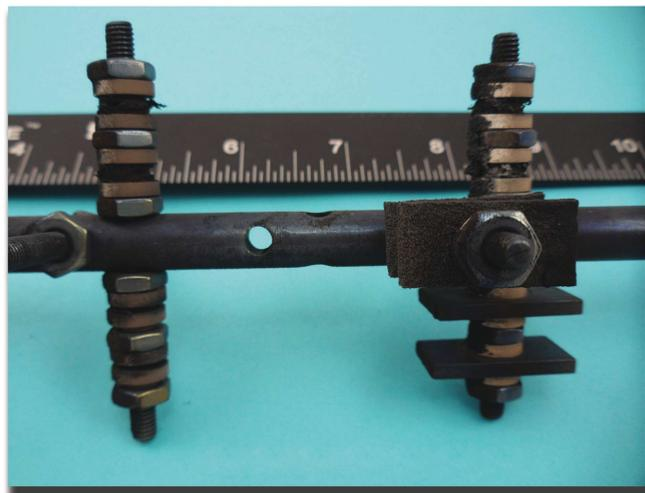
A view of the specimen rack following exposure to the aggressive acidizing environment. The Type 316L SS coupons on the upper right side of the rack and titanium alloy coupons on the left side of the rack were completely dissolved. Photo courtesy of Honeywell Corrosion Solutions.
