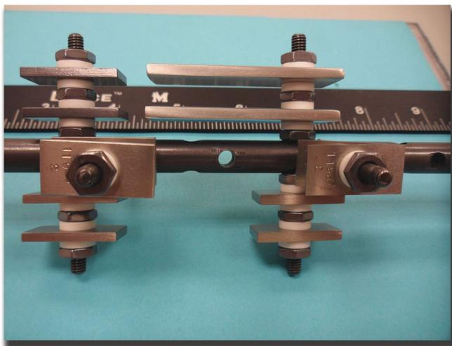
A view of the Ta-surface-alloyed specimen rack before testing in the mild acidizing environment. Photo courtesy of Honeywell Corrosion Solutions.
