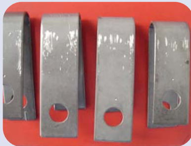
Fig. 6b — After being coated with Tantaline, parts can be bent to a U shape with an undamaged surface.
