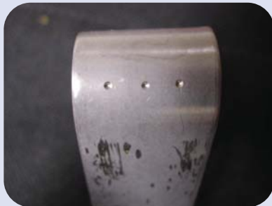
Fig. 6a — Sample coupons were indented with a Rockwell C cone shaped hardness indenter to create localized stress upon the surface.
