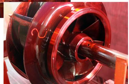
There are two basic types of penetrant examination. A visible penetrant is usually red in color and produces vivid red indications in contrast to the light background of an applied developer under visible light (see Figures 1 and 2). The fluorescent penetrant, usually green in color, fluoresces
