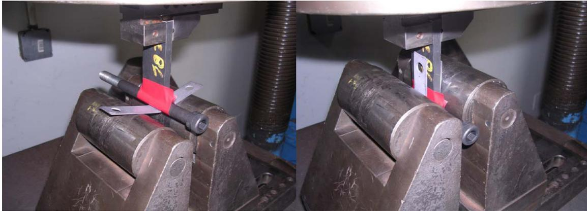
Figure 3. U-bending over 3/8" mandrel. Rockwell indentations are at centre of strip on lower side experiencing tensile deformation.<sup>[1]</sup>
