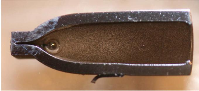
Figure 4: Cross section of thermal shock test specimen. After 100 water quench cycles from 300 °C no crack or signs of deterioration is seen.
