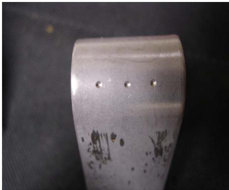
Figure 5: Ruggedness test coupon indented with Rockwell C and U-bent over 3/8" (10mm) mandrel.<sup>[1]</sup>
