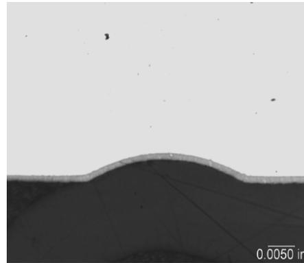
Figure 6: Micrograph showing uniform deformation of substrate and tantalum surface alloy at indentation. No cracks or delamination is seen.<sup>[1]</sup>
