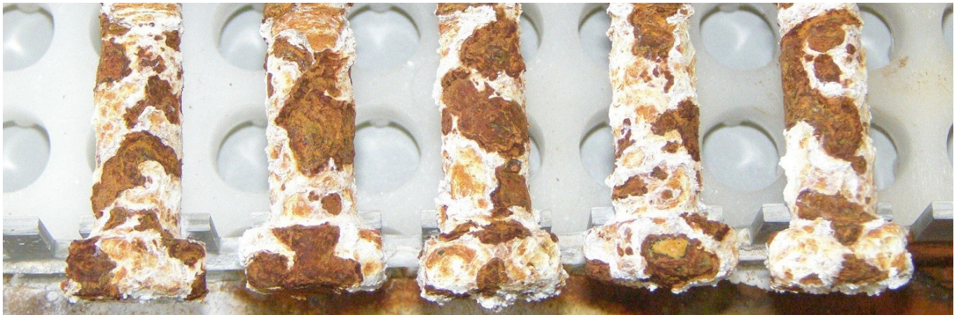
Heat zinc galvanized bolts after 12 week test.
