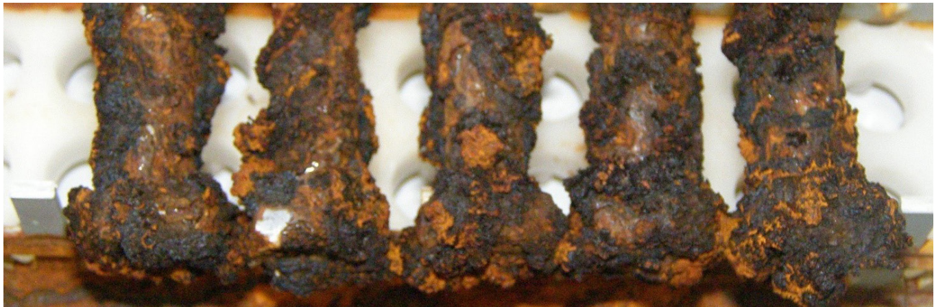
Zn electroplated and Cr III passivated bolts after 12 week test.
