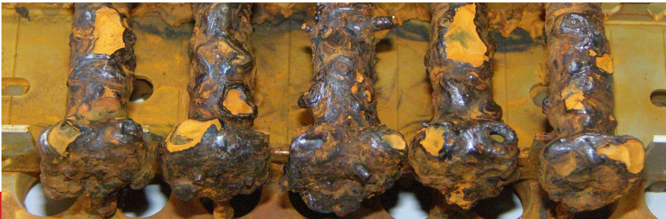
Untreated bolts with oil-film protection, after 12 week test.
