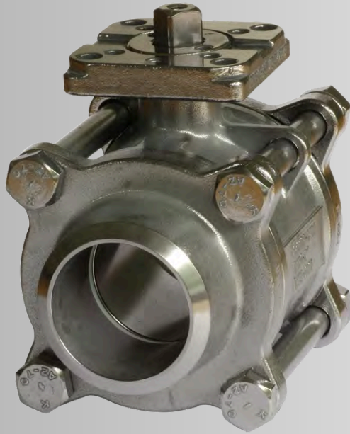
Treated with Tantaline® after 48 hours in hot acid
