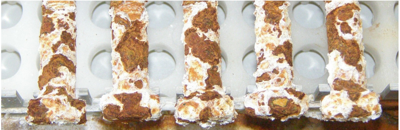
Hot zinc galvanized bolts after 12 week test.
