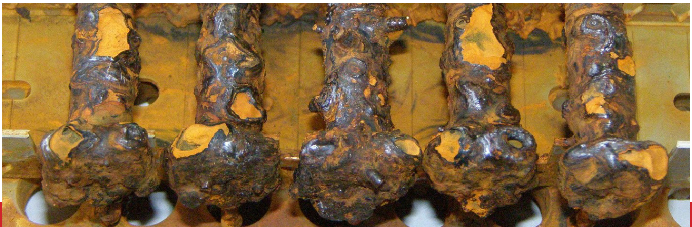
Low carbon steel untreated bolts with oil-film protection, after 12 week test.
