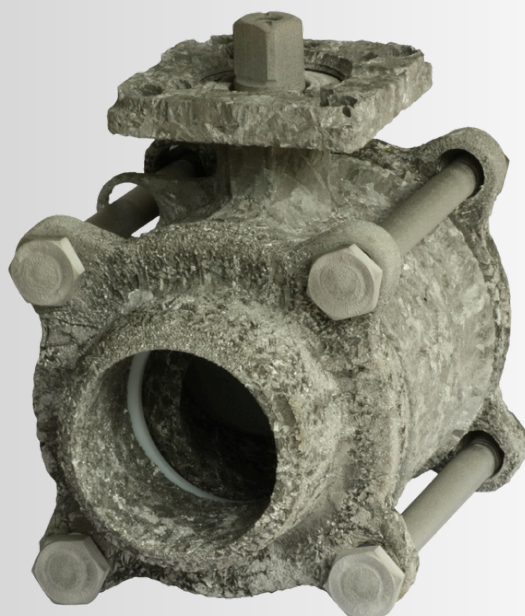
Untreated after 10 hours in hot acid
